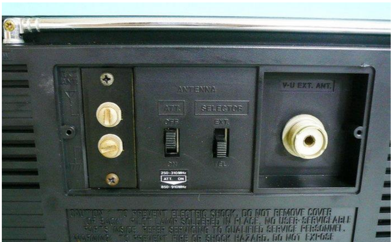
Figure 15: The label placed under the antenna attenuator switch of the Japanese version of the NR-108F1 receiver
