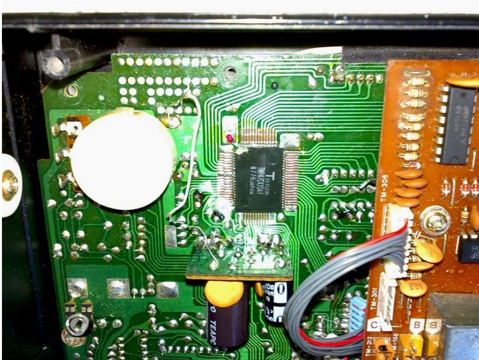
Figure 13: The Toshiba TMP47C420AF main processor of the NR-108F1 (shield removed) [5]
