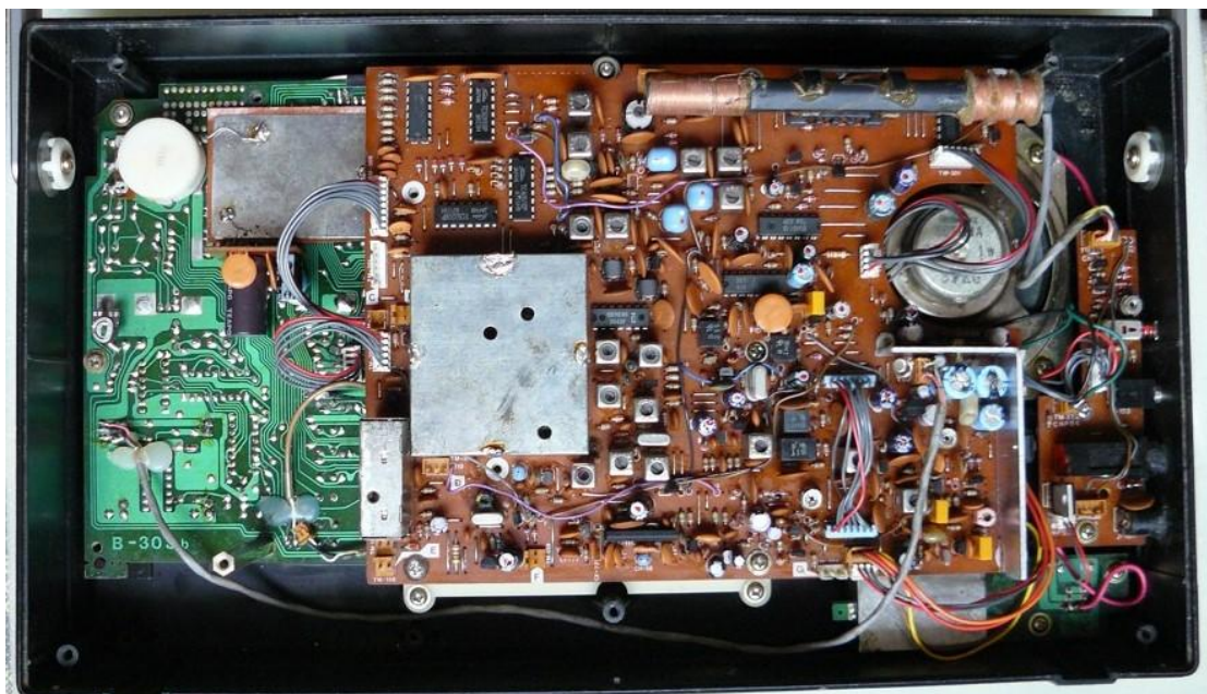
Figure 12: A NR-108F1 with the V-UHF tuner removed [5]
