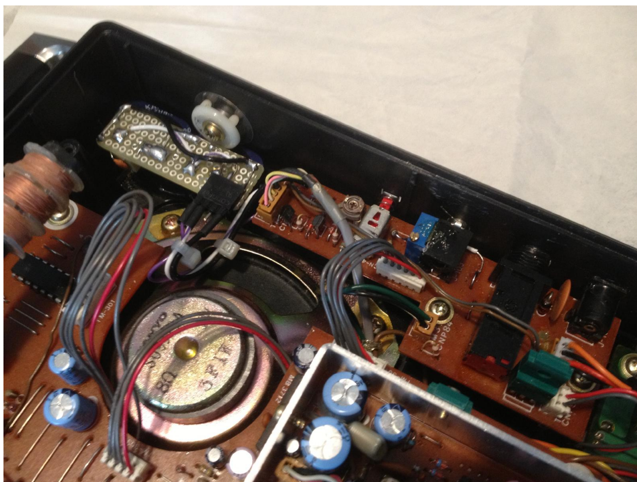
Figure 20: Location of the added board and of the multi-turn resistive trimmer
