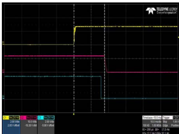
Figure 7: DS495SPE-3 Turn Off Characteristic via PS_ON_L Full Load: I_O = 41.25A Ch 1: PS_ON_L Ch 2: V_O Ch 3: Pwr_Good
